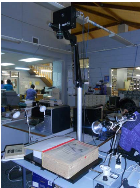
The microfilm camera set up for copying large bound volumes of The Samoan Times in the NUS Library workspace.
